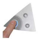
To exit the menu, press and hold the Main Button for 2 seconds.
