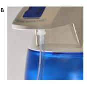
Push one end of the Tygon Tubing onto the end of the Barbed Fitting (B).
