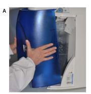
• Open the front cover (this may require to remove the final filter) to go into STANDBY mode (A).
