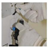
• Ensure that you use the gloves supplied with the UV replacement kit. Plug the electrical cable to the new UV Lamp (H).
